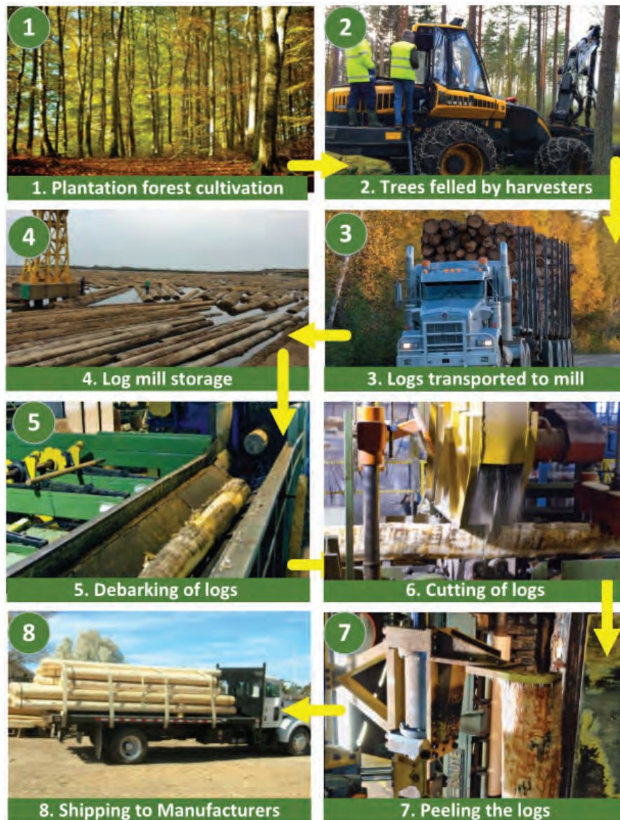
Figure 18.5. Steps in Modular (Knockdown) Furniture Manufacturing
